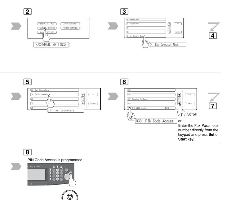
• To return the machine to the initial screen of the current
